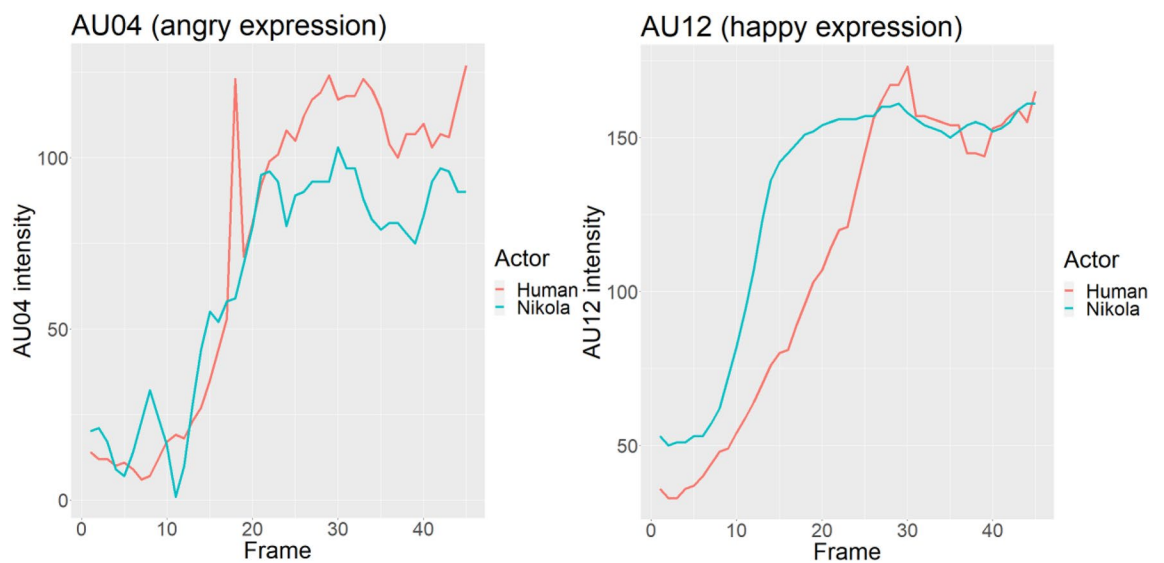
Figure 5. Trajectories of AU04 (brow lowerer) and AU12 (lip corner puller) intensities across video frames, for human and android expressions.
